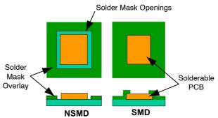
Figure 8. Comparison of NSMD vs. SMD Pads
