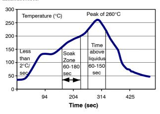
Figure 11. Typical Reflow Profile Lead Free Solder
