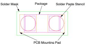
Figure 4. Recommended Mounting Pattern
