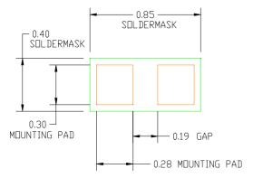
Figure 6. Recommended Mounting Pattern
