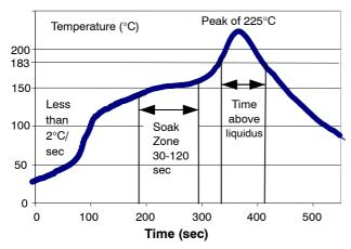
Figure 12. Typical Reflow Profile Eutectic Tin / Lead Solder
