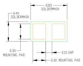
Figure 7. Maximum Recommended Mounting
