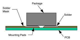
Figure 5. Cross-Section of Mounted Package
