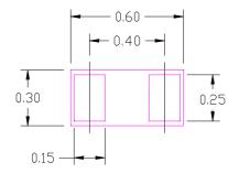
Figure 2. Dimensioned Bottom View of Package
